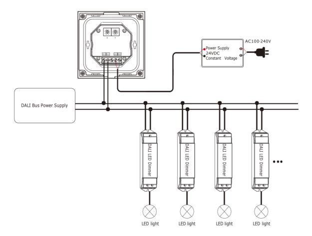
Note: It is recommended to use a 24VDC power supply for the touch panel DALI master to reduce the load on the DALI bus power supply.
